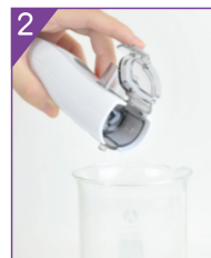
Open the medication cup cap and pour out any remaining liquid.
